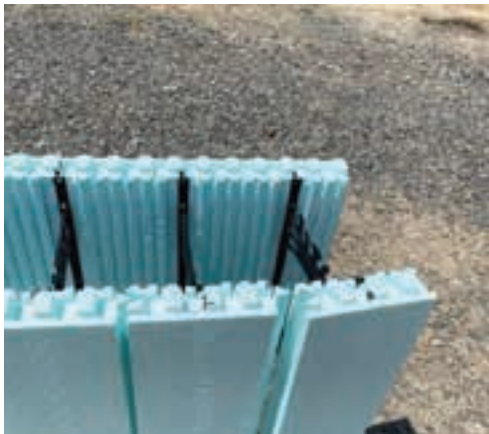
Insulated Concrete Forms (ICFs).
